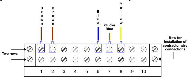
The recommended gauge for Status/Control connection wires is 16 AWG - 600VDC (1.3mm<sup>2</sup> wire section). Wire size and installation must comply with all applicable local, regional and national regulations (e.g., National Electric Code for USA).
